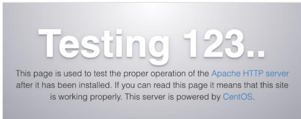
This page indicates that Apache is working correctly. It also includes some basic information about important Apache files and directory locations. Now that the service is installed and running, you can now use different `systemctl` commands to manage the service.
