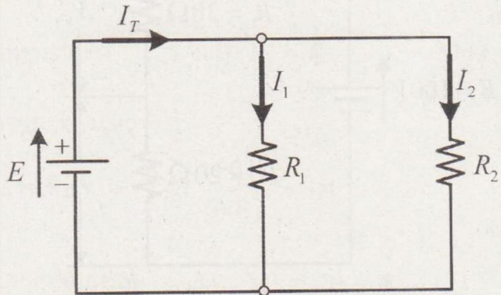
$$I_1 = I_T \frac{R_T}{R_1} = \frac{I_T R_2}{R_1 + R_2}$$
