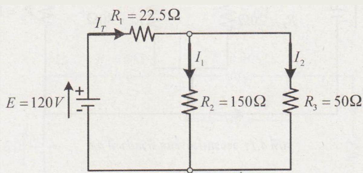
$$R_{Tl} = \frac{R_2 \times R_3}{R_2 + R_3}$$
