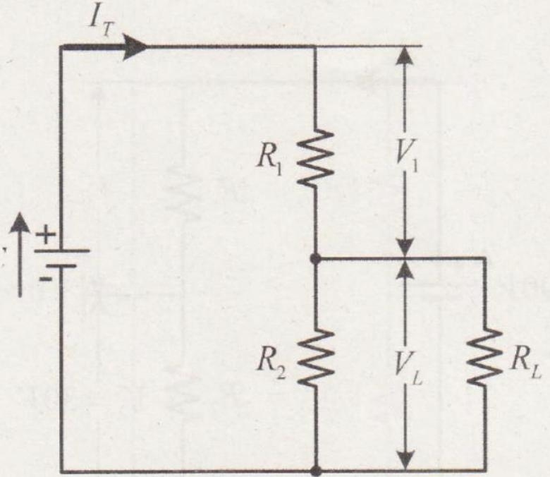
$$R_T = R_1 + (R_2 // R_L) = R_1 + \left( \frac{R_2 \times R_L}{R_2 + R_L} \right)$$
