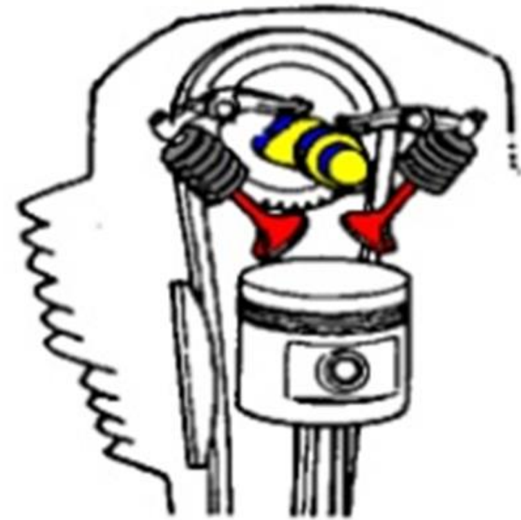
SOHC Single Over Head Camshaft
