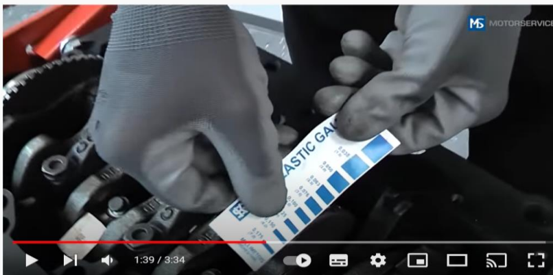
Measure bearing clearances with the KOLBENSCHMIDT PLASTIC GAUGE - Motorservice Group
