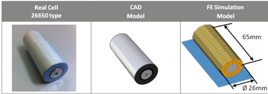
Fig. 2.6 Picture of a cylindrical cell with an aluminium casing ( left ), the CAD model of the cell ( middle ), and the FE model ( right )
