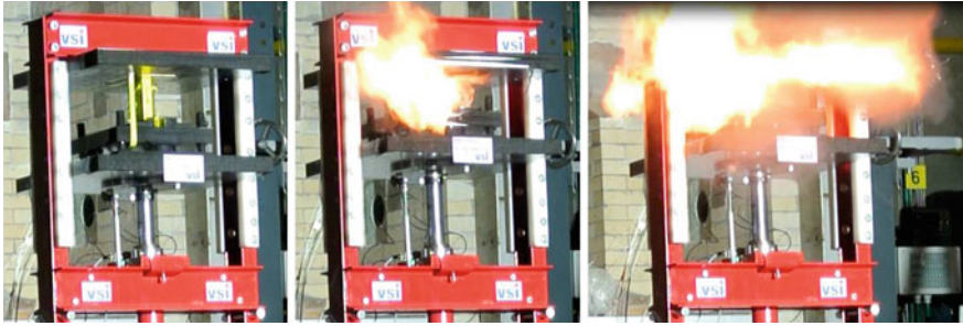
Fig. 2.1 Exothermal reaction of a single charged cell under severe deformation—test conducted in cooperation with TU Graz, Vehicle Safety Institute
