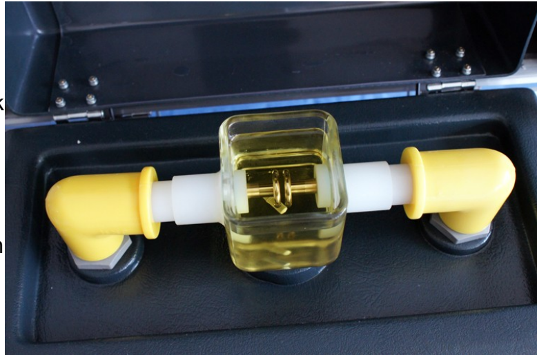
Illustration 1: Dielectric Strength Testing of Coolant
