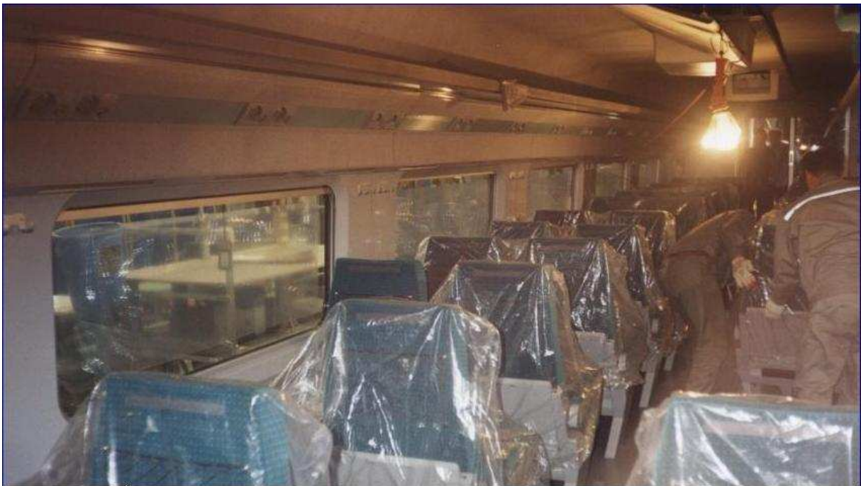
Seats being installed inside coach body.
