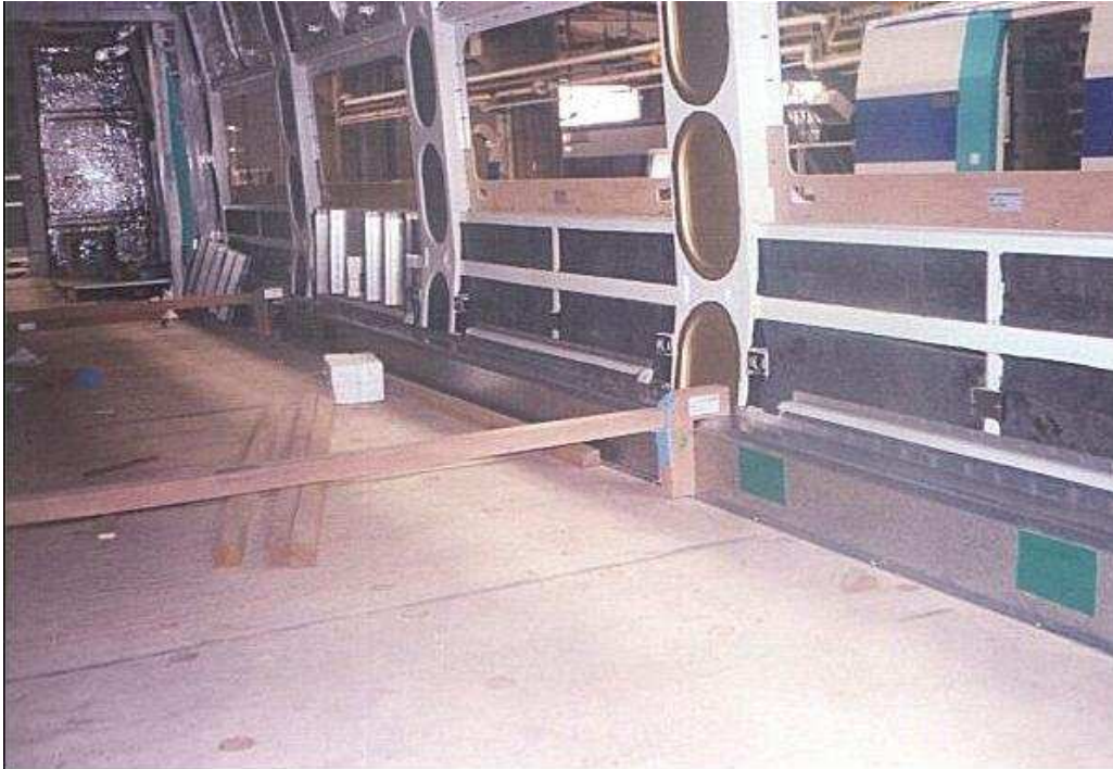
Interior of TGV trailer. On the car wall between the windows you can see large oval brass coloured inserts. These seal the area after the sound deadening material has been added. At the base of the windows is a jig that is used to protect the car shell during the installation of the window frame. In the right foreground is the wooden jig that holds the floor level HVAC ducting in place ready for fixation. Some of the sound deadener can be seen in the rear and car ceiling.
