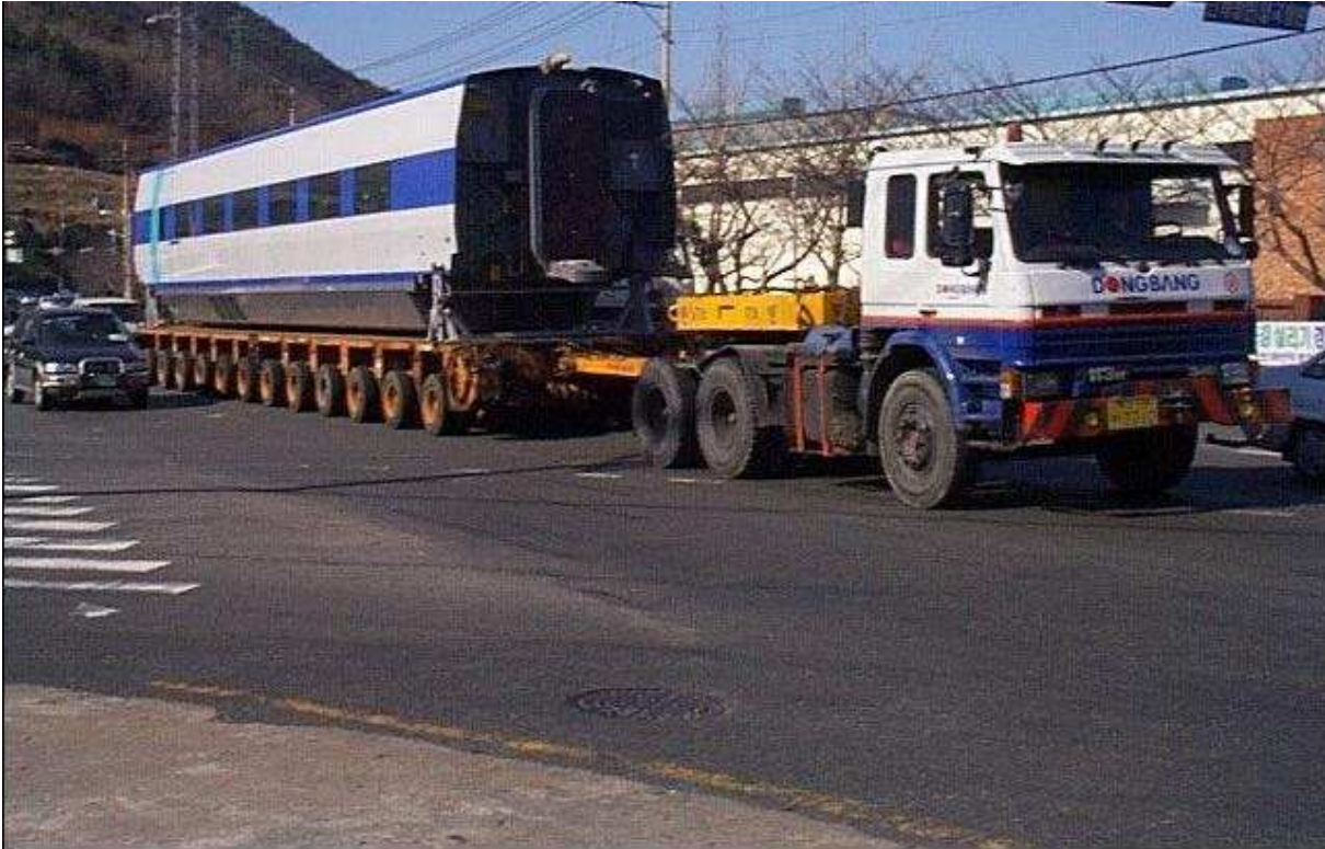
A TGV high speed vehicle being moved through the streets to the factory where it will be reunited with its bogies. The vehicle has been lifted off the special trailer used during shipping and placed on to a road trailer as seen here. The route taken by road will have been surveyed to ensure that there are no obstructions like telephone wires and traffic signals which could be damaged. Note that the body corners are supported on jacks to prevent the underframe equipment being damaged by the weight of the car body.
