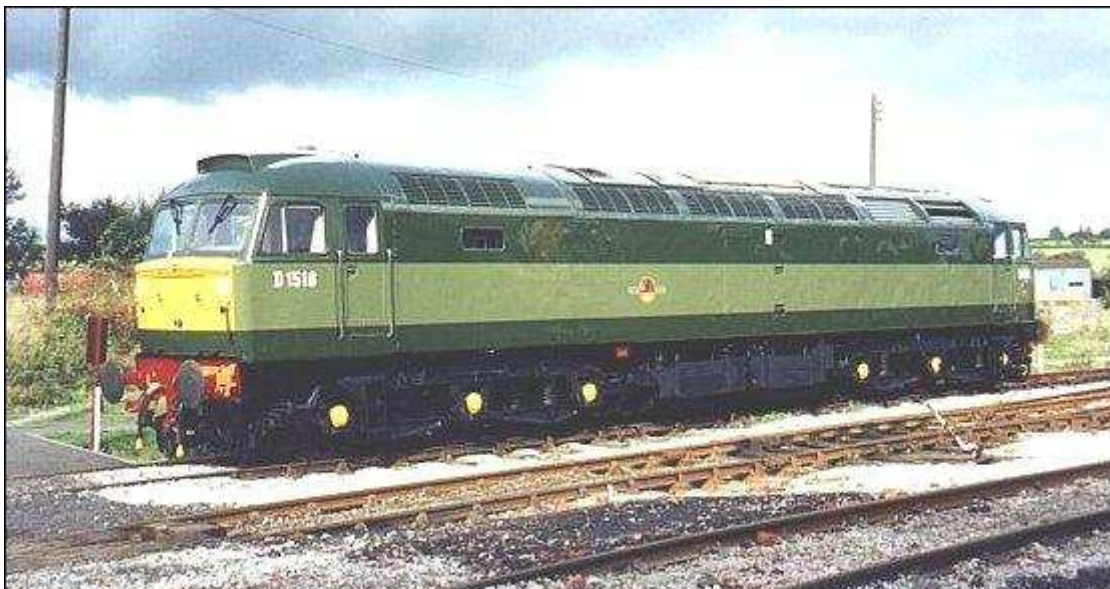
The UK Class 47 Co-Co diesel-electric locomotive, first introduced in 1962 and still regularly seen all over the country. The original engine was built to a Sulzer design and is a 12 cylinder, double bank machine rated at 2580 hp.
