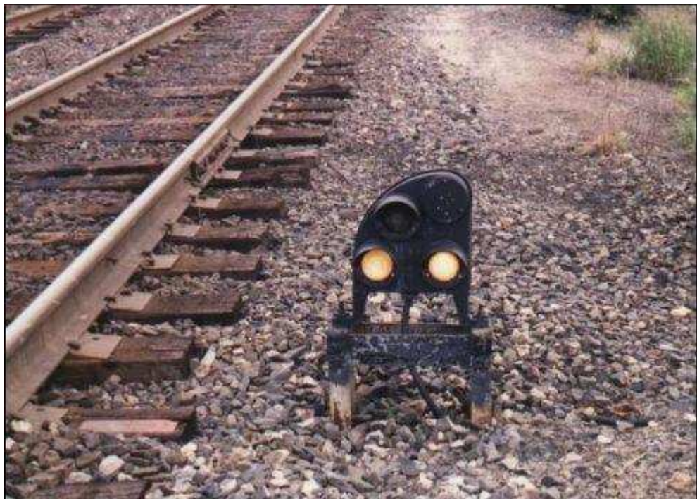
US position light dwarf signal capable of showing "stop" (as seen) and "restricted speed". This signal bears a strong resemblance to the UK shunt signal.
