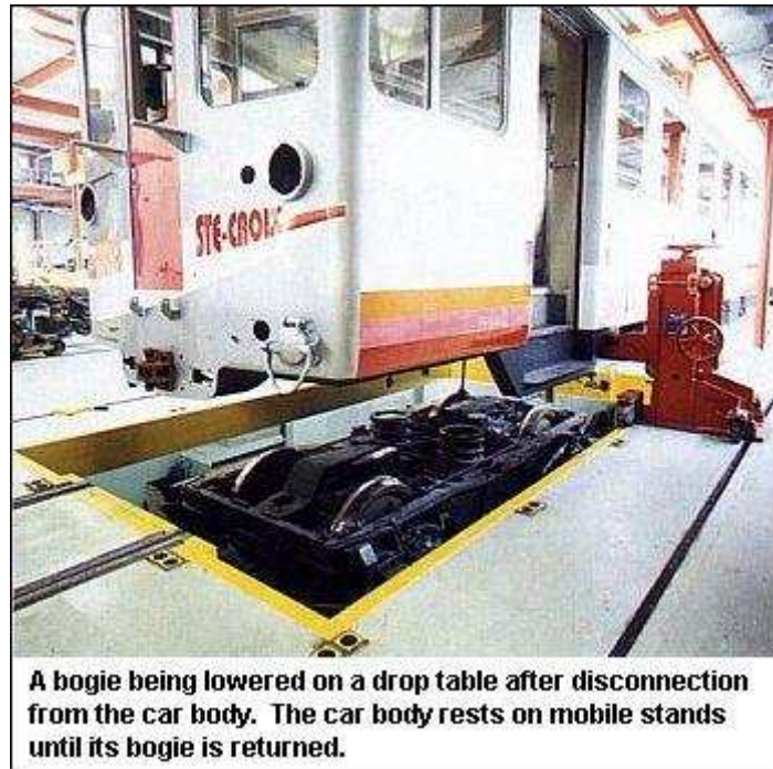
Bogie being lowered
