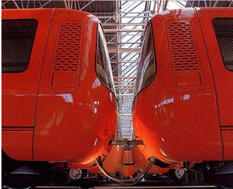
Two cars of a metro EMU unit used in Lyons, France coupled with a bar coupler. This type is bolted in the centre, other types are solid with a removable connection under the car body. The electrical and pneumatic connections are carried in the cables hanging under the coupler bar.
