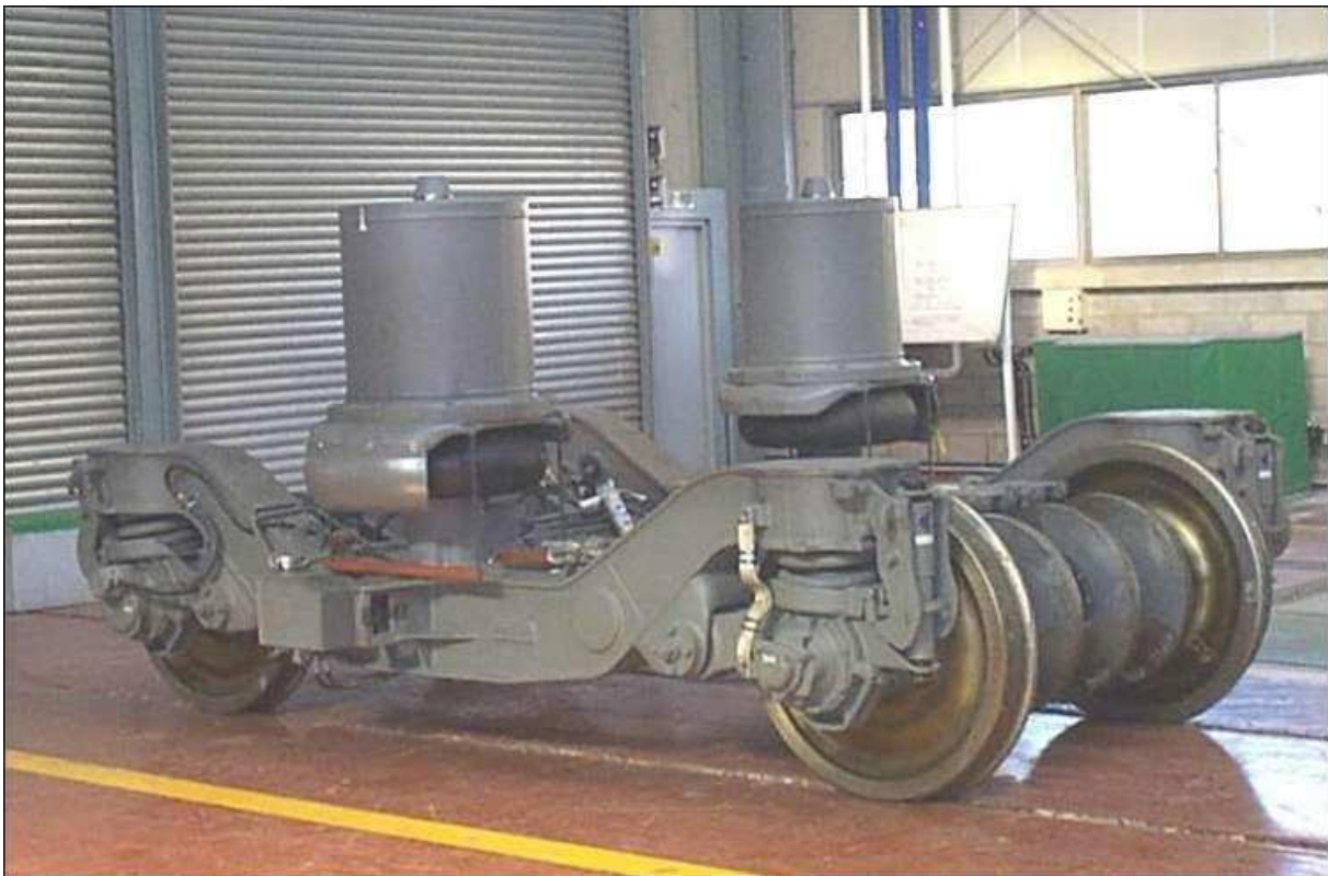
Trailer bogie for Korean TGV high speed train. The large suspension units support the articulation between the two adjacent car bodies. Note the provision of 4 large braking discs on the axle to cope with braking from high speeds.
