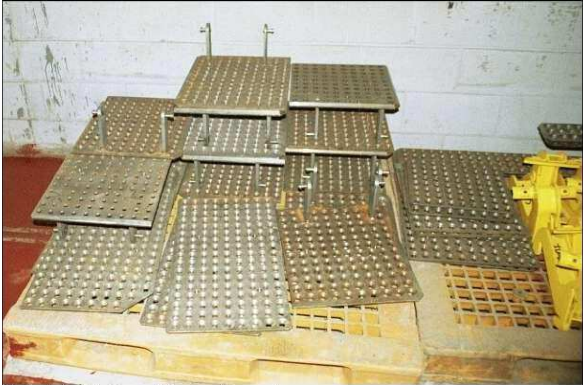
Bodyside straightening panels for use with magnet.
