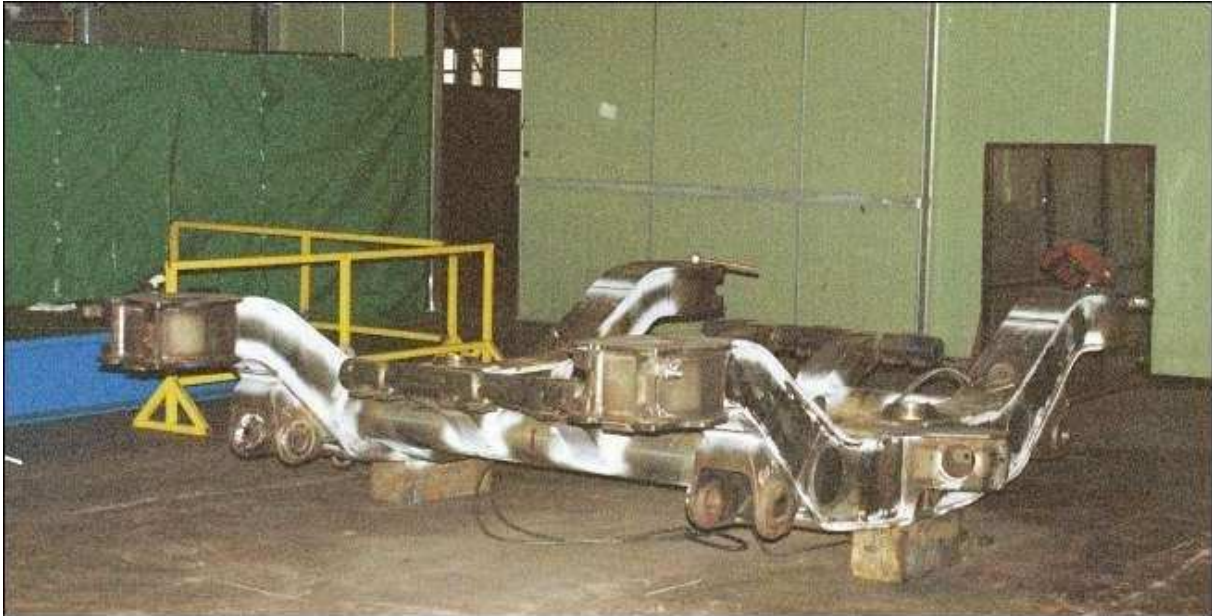
Bogie frame after welding and before painting. The white marks are dye penetrant for non-destructive testing.
