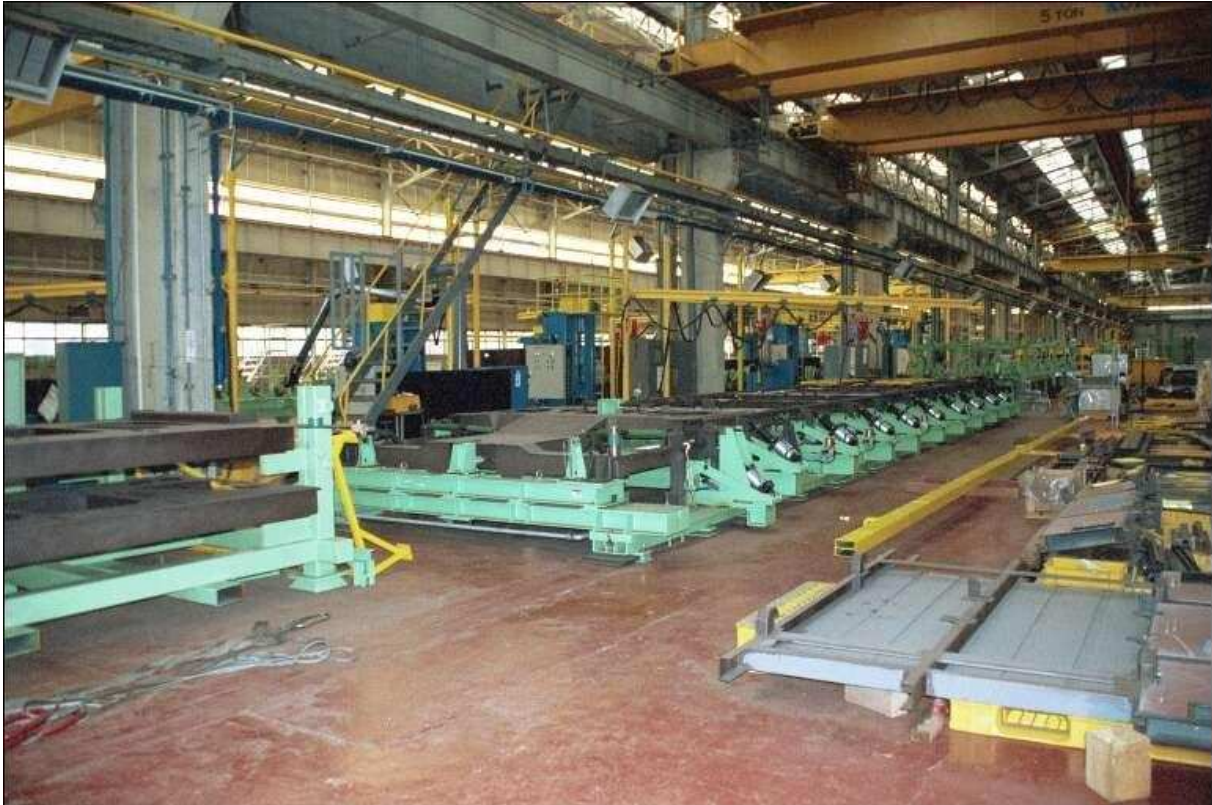
Underframe inverted in assembly jig where the bolsters are added and camber will be introduced.
