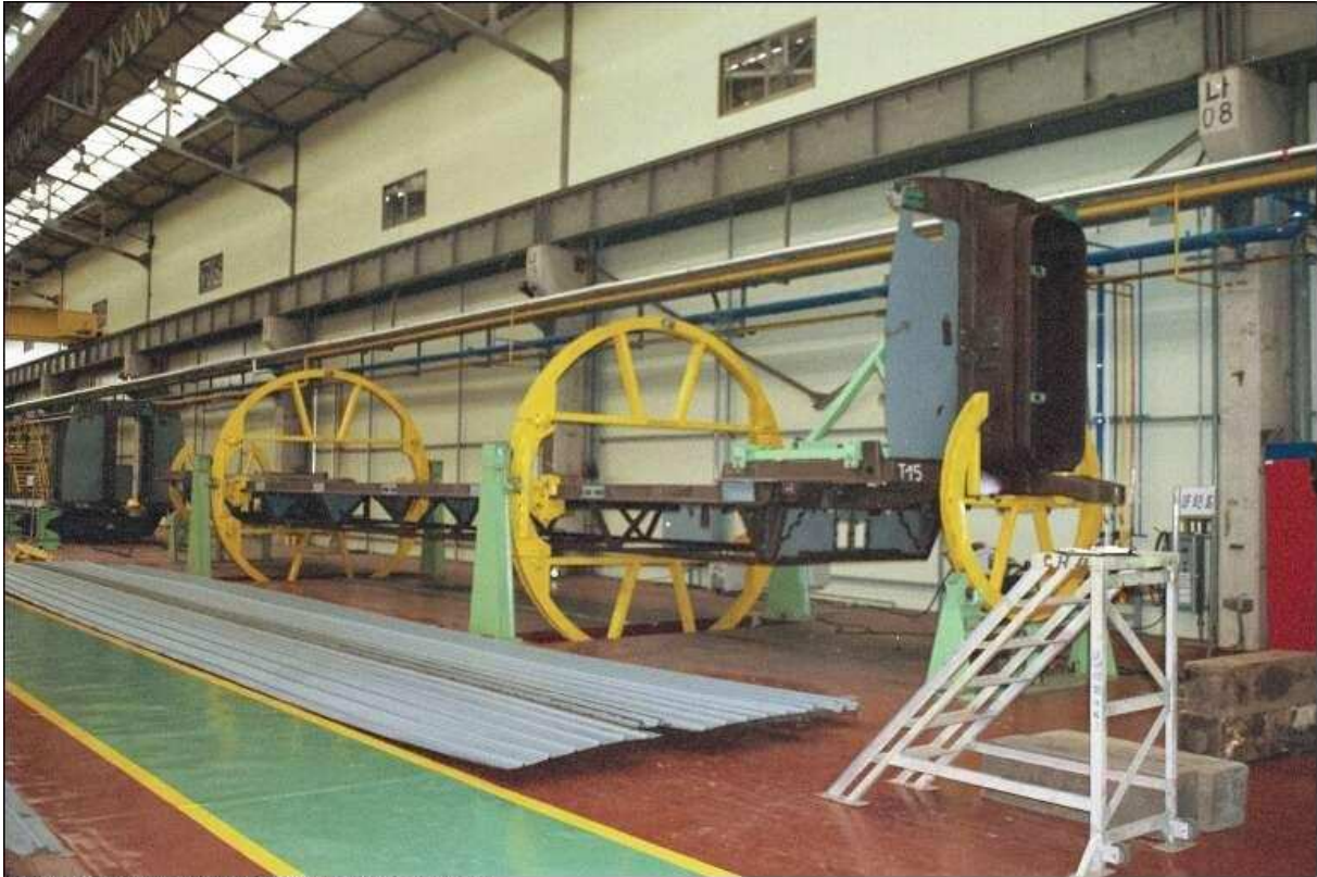
Underframe in rotating jig with car end welded on.
