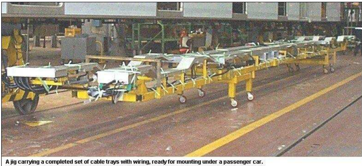
A set of cable trays ready for fitting
