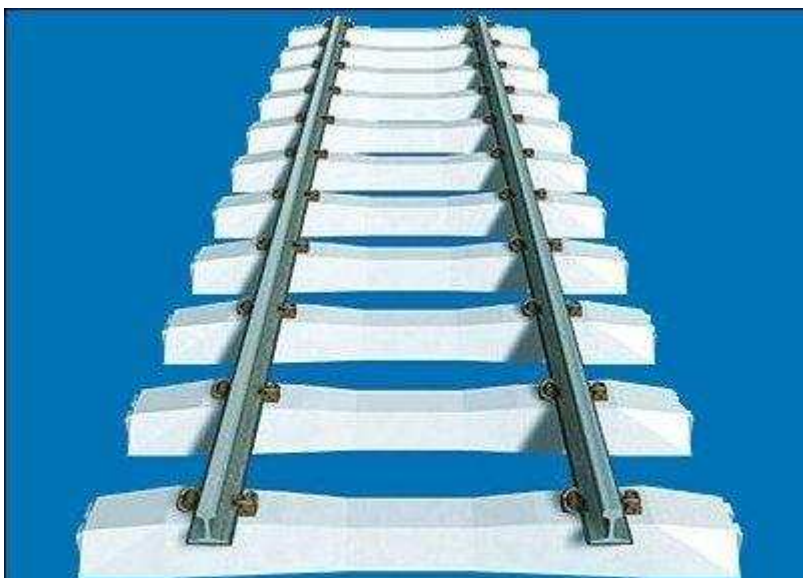
Typical arrangement of concrete sleepers with flat bottomed rail and pandrol clips. Note how the sleepers are shaped to provide a degree of natural drainage.
