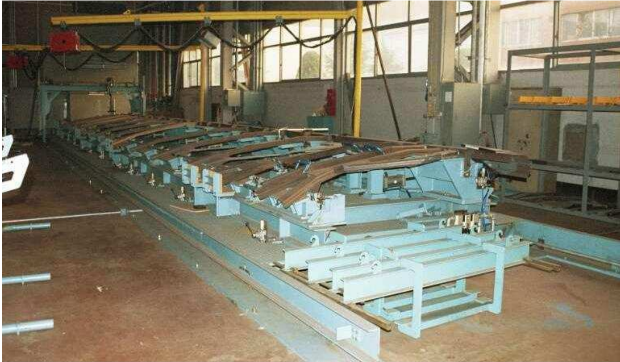
Body-side assembly jig. It is shaped to match the body curvature. The panels and their internal strengthening members are held in place by clamps while being welded.
