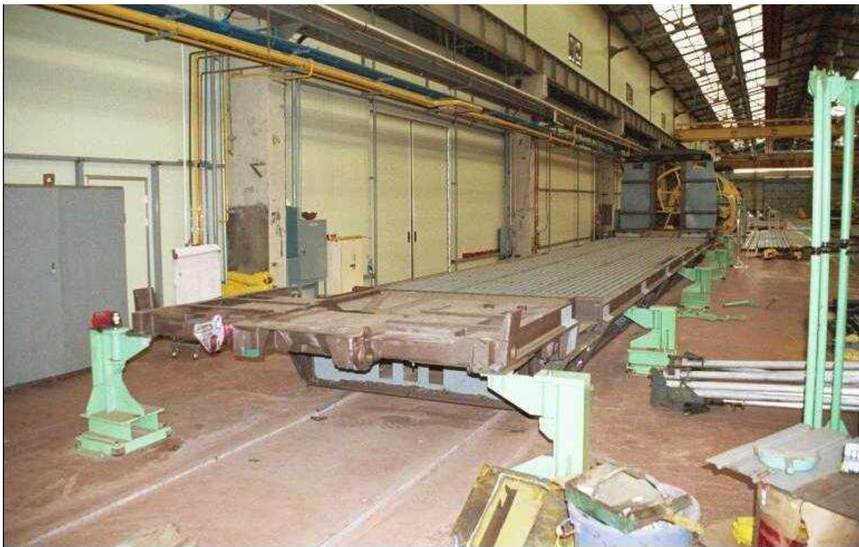
Underframe and car end completed.
