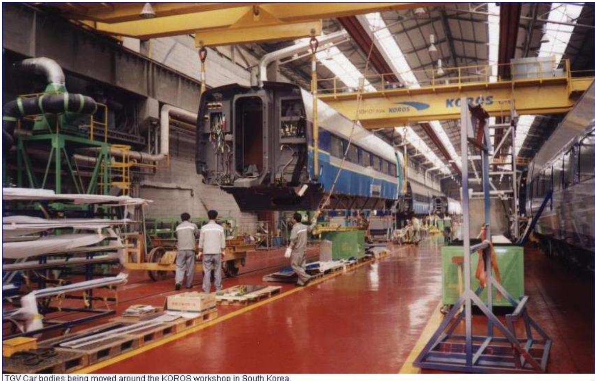
TGV Car bodies being moved around the KOROS workshop in South Korea.
