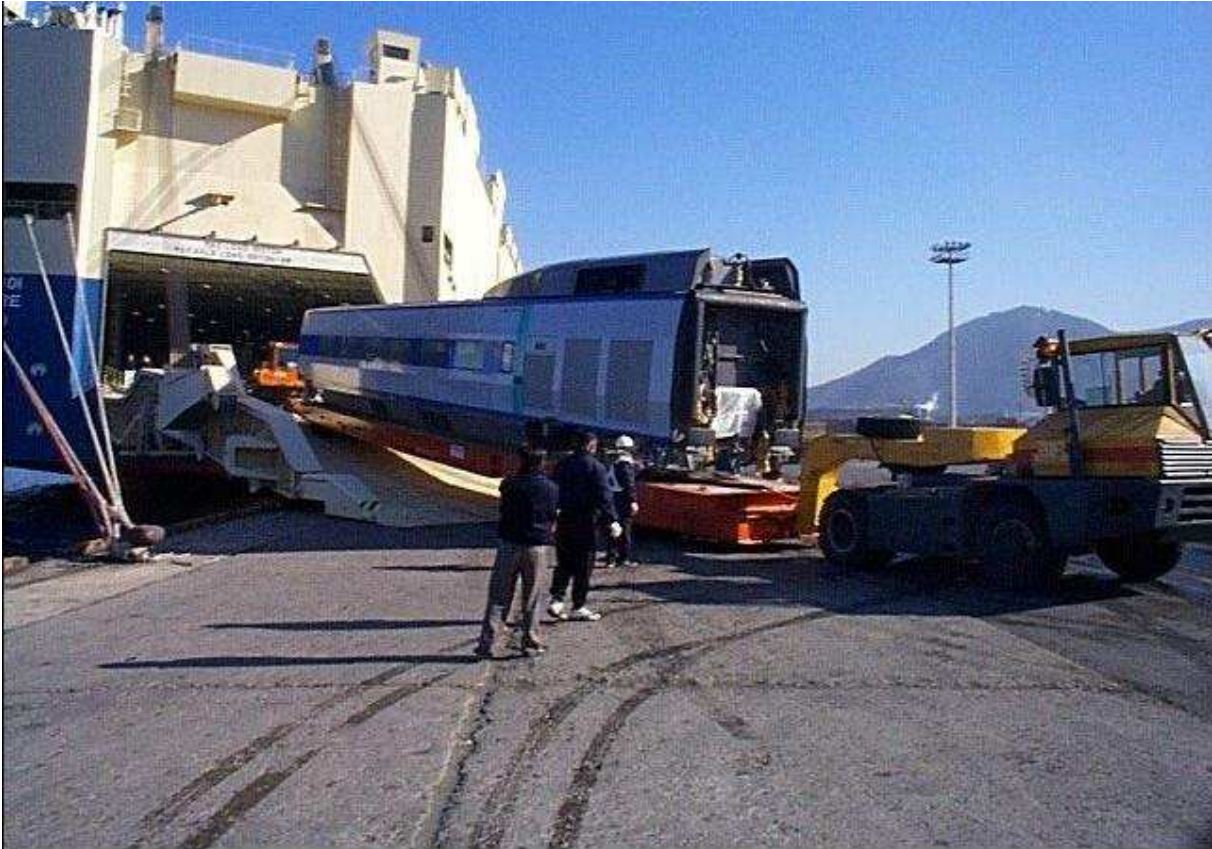
A TGV high speed vehicle being unloaded from a car ferry ship in Korea. The move from the deck of the ship is a delicate operation carried out using a special trailer and tractors.
