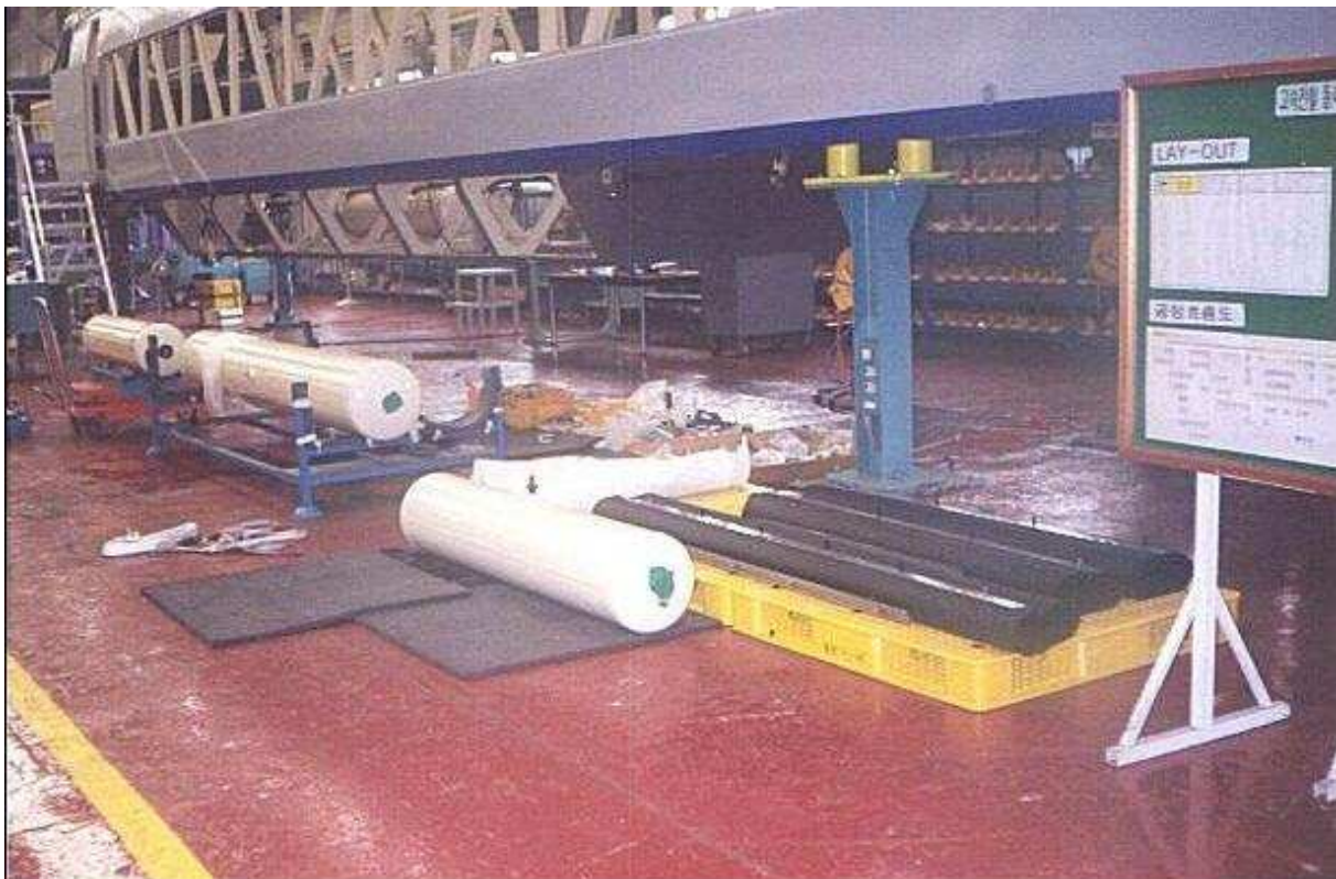
TGV power car awaiting the fitting of air reservoirs for the braking system. One has already been fitted while the remainder are lined up on the shop floor, ready for mounting.
