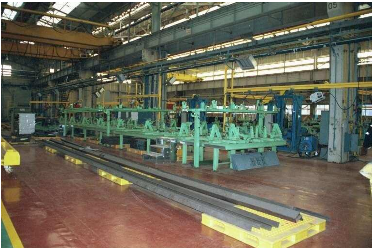
Underframe assembly jig, where all the parts are laid out and welded into place.
