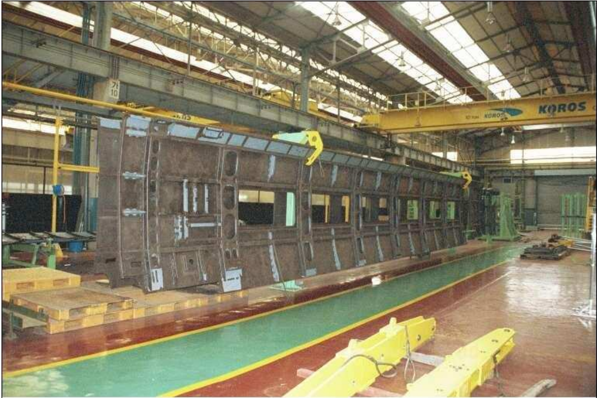
Bodyside ready for transfer to bodyshell assembly jig.
