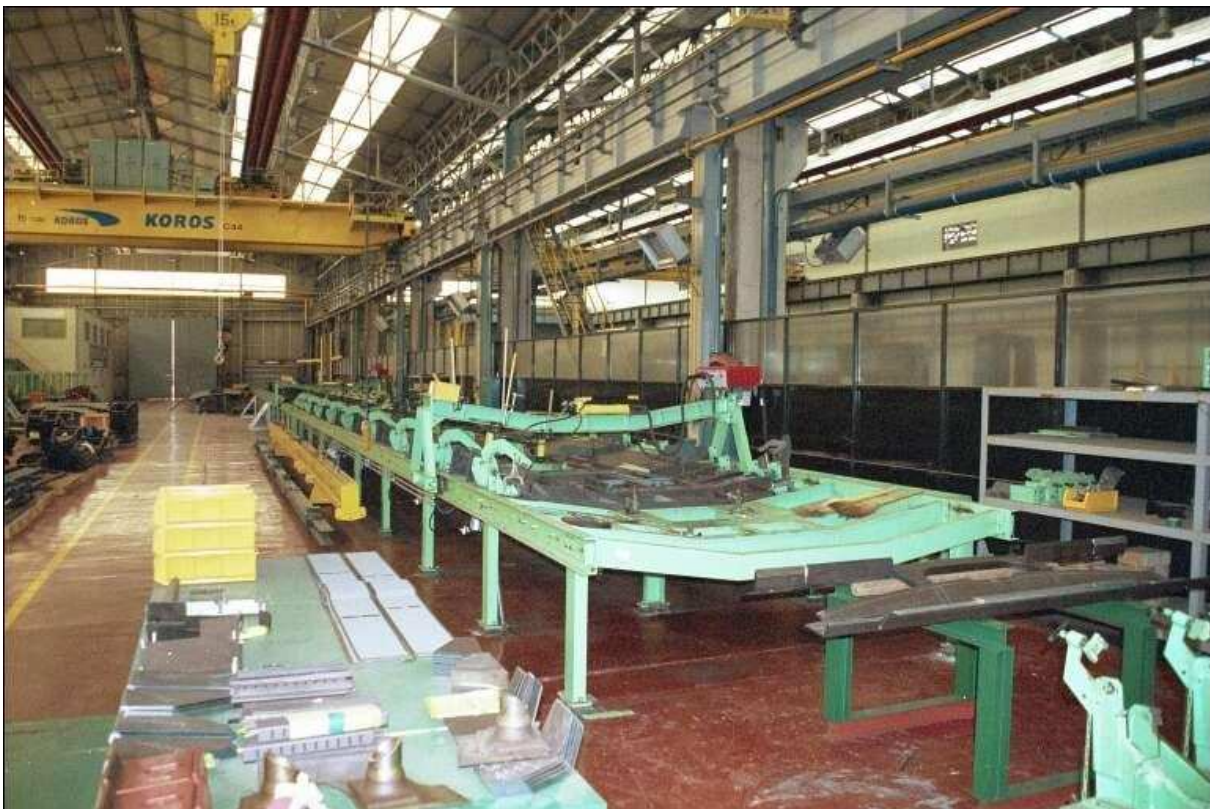
The roofing jig, where the parts are clamped to provide stability during welding. The roof is one of the more difficult parts of the car to weld as it is thin and tends to distort easily.
