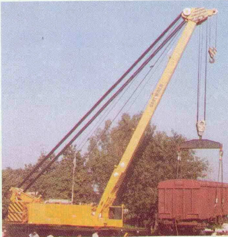
140 t Crane, 285 hp (1986)
