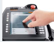
Efficient operator control with brilliant, capacitive touch display. Input the 8.4" screen.
