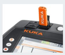
State-of-the-art hardware. Thanks to the latest hardware, the KUKA smart-PAD will impress you with its strong performance. Two easily accessible USB ports enable direct saving and loading of application programs and connection of
