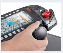
Simple robot jogging with the ergonomic 6D mouse. It offers intuitive jogging and reorientation of the robot in can be made quickly and easily via three or six degrees of freedom.
