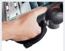
Comfortable, relaxed handling. The KUKA smartPAD features impressively pleasant handling. Straps and handgrips that can be used with both hands greatly ease operator control. An optional shoulder strap enables the operator to work without tiring – particularly during other supported USB devices. time-intensive projects.
