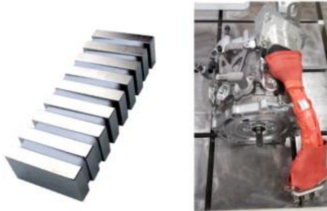
รูป 4-11 (Left) An example of a sintered NdFeB magnet and (right) the 80 kW interior permanent magnet motor from the Nissan Leaf, in which such magnets are use [5.19]
