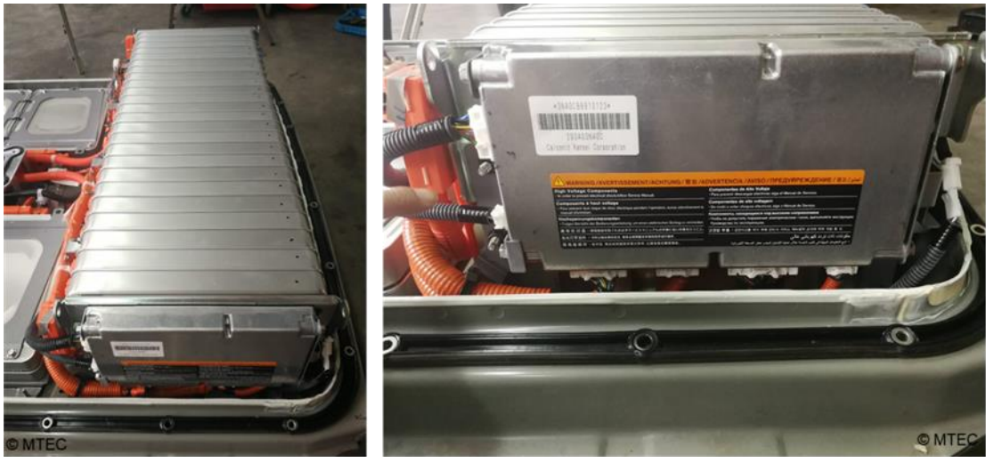
รูป 3-42 Battery Controller
