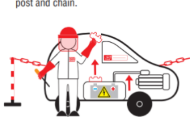
Face shield, insulating gloves, voltage detector, padlock, safety boundary post and chain.
